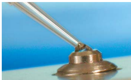
Pipetting 1 µl onto optical surface
